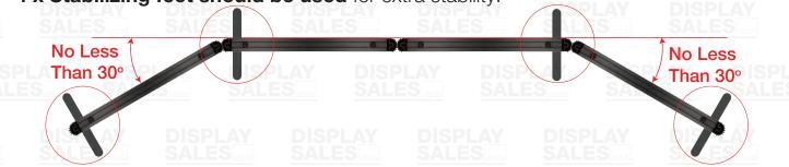
When using the folding panel system in the following configurations,
